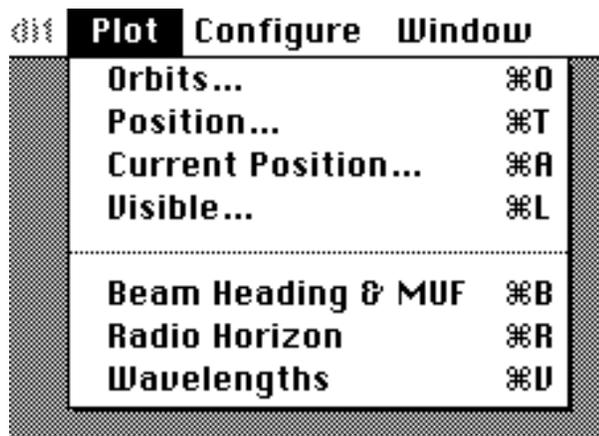
A maximum of 5 orbit and position windows may be open. Orbit windows may contain a maximum of 32K of information each. Any orbit plot which attempts to exceed this limit will be terminated with a warning when the limit is reached.
