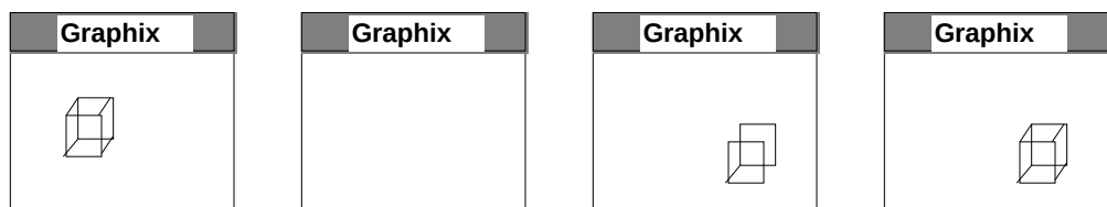
fig II.OS1: The animation cycle (from left to right). The old image is first erased and then redrawn. On slow machines this will produce flicker.
