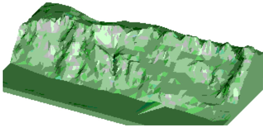
fig IV.1: Churfirsten (part of a mountain range in Switzerland) drawn with GeoBench/GrafSys using Triangulation.
