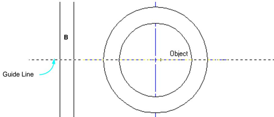
6. Move to the intersection of the horizontal centerline and the right center of the body (Arc End cue) then downwards without clicking. When the **Offset/ Align H** cue appears click.
