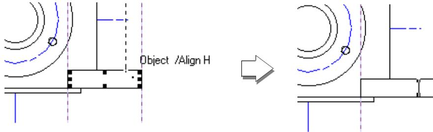
17. In the Top View drawing, use the Center cue to find the left end of the guideline in the right lower ear. Move to the left until the Object/ Align V cue appears then move downwards.
