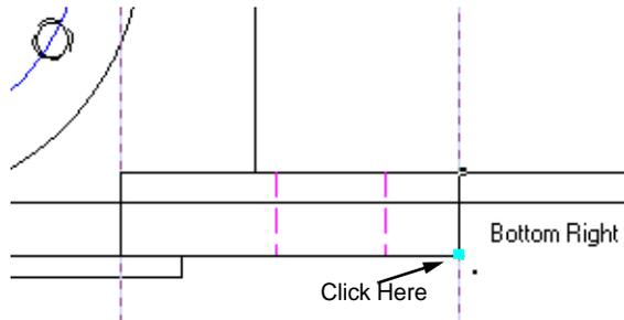
8. Find the bottom right of the lower most rectangle (Bottom Right cue) and click. Draw a horizontal line that ends around the same distance as the previous line then click.
