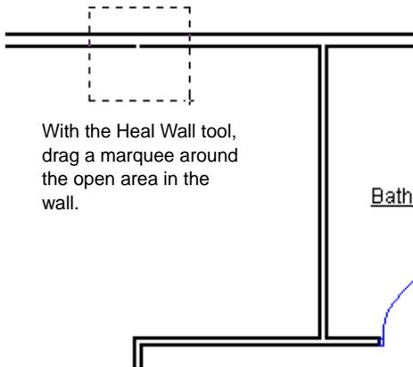
With the Heal Wall tool, drag a marquee around the open area in the wall.
