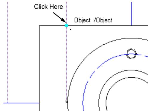
11. Move downwards then press the Tab key until the delta Y field is highlighted. Enter **-15** and press the **Enter key**.
