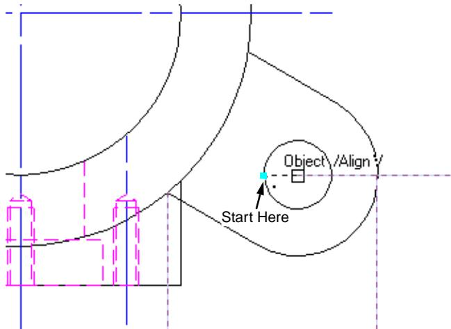
18. With the Align H cue active, move down until you reach the top of the rectangle just drawn in the Front View (Object/ Align H cue) and click. Draw a vertical line extending to the bottom of the rectangle (Object/ Vertical cue). Click to end.
