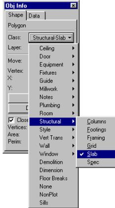
This changes the class the polygon is in. Choosing a class or layer from the Object Info palette changes the layer or class an **Object is in**. Choosing a layer or class from the pulldowns on the Data Display bar changes the layers or class that you are **currently viewing and drawing in**. This polygon represents the slab.
