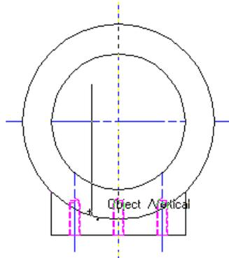
7. Move the cursor over the large vertical centerline. Press the **T** key.
