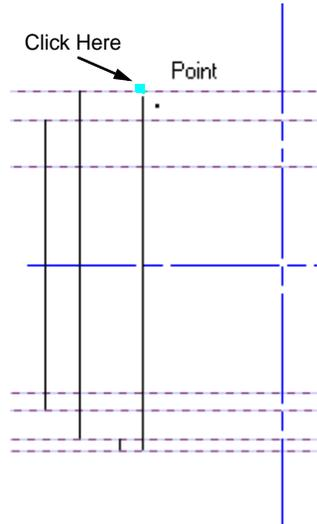
3. Moving in the left direction, trace the outline of the four vertical lines as shown.
