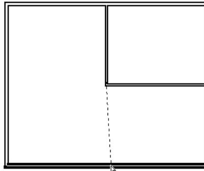
The short vertical wall is extended the full width of the house and is joined correctly at top and bottom. The interior connection has been changed and needs to be joined.
