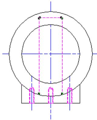
22. Click on the horizontal centerline. Hold down the Shift key and click on the two vertical lines.
