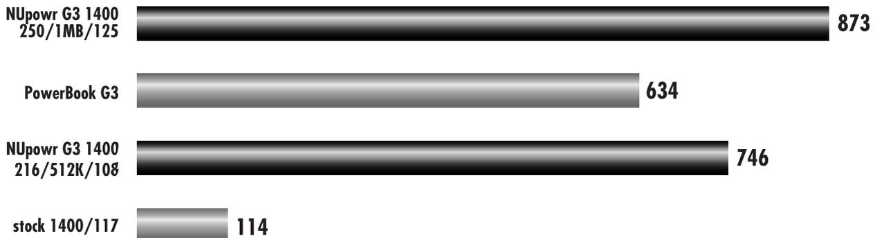
The magic of the PowerPC 750 chip is its ability to talk to the "backside" cache memory on the processor card at high speeds - up to the same speed as the clock of the CPU. The high number of cache "hits" makes the speed of the system bus almost irrelevant because the data is read from the cache memory at speeds far faster than the slower system bus.
