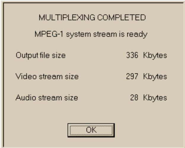
Here is an example of the **final message** box. It shows the output file size, video stream size, and audio stream size in Kbytes.
