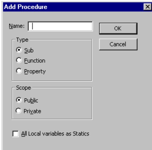
Inserts a new Sub, Function, or **Property** procedure. The **Add Procedure** dialog box also allows you to set the scope to public or private, and make all local variables in the procedure static.
