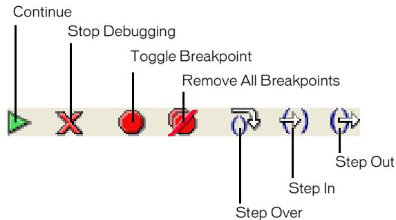
**Step In** advances the Debugger (indicated by the yellow arrow) into a function. Step In works only for user-defined functions.
