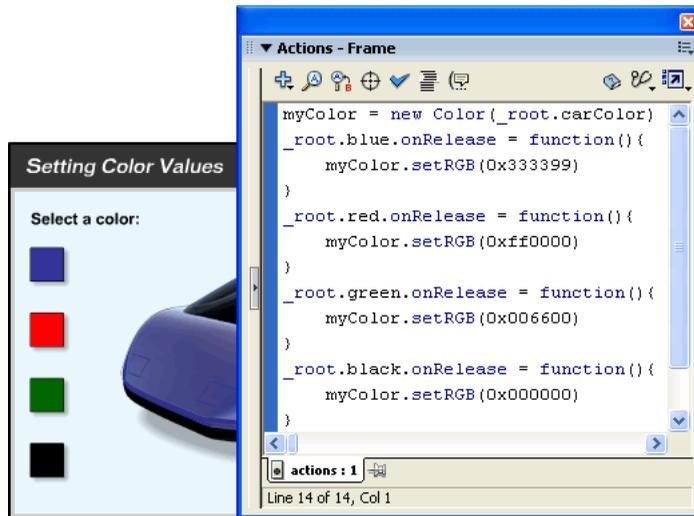
*The button action creates a Color object and changes the color of the car based on user input.*
