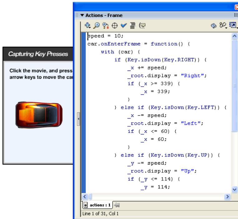
*The input from the keyboard keys moves the car.*
