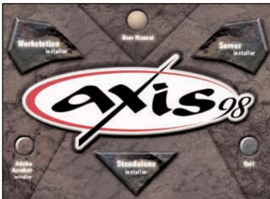
When the CD ROM is inserted, it should autoplay, and after a few seconds you should see the Axis 98 InstallPad Window. If you have autoplay turned off, or it doesn't start for some reason, look inside "My Computer" and open the CD ROM manually. Then double-click (run) the file "InstallPad.exe".
