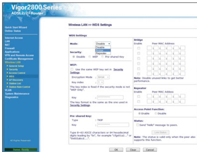
Routers and access points that support the Wireless Distribution System can be configured as wireless bridges/repeaters, but it's complicated and not a common option
