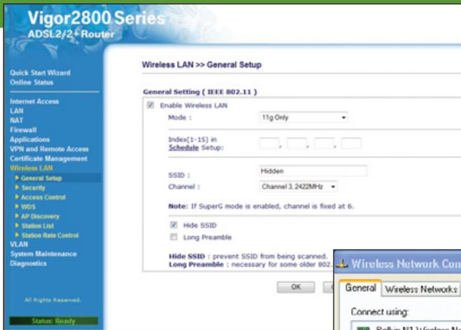
Disabling broadcasts of the network name (SSID) may seem like a good security measure, but it's easily bypassed and can cause connectivity problems
