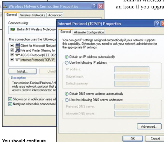
You should configure wireless clients to get an IP address automatically from the DHCP server
