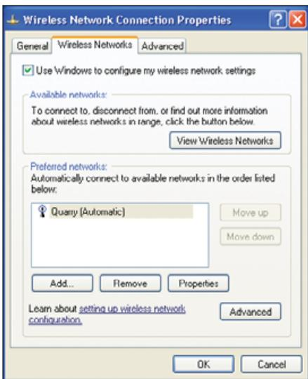
Most adapters can be managed using either vendor-supplied software, or the tools that are included in Windows
