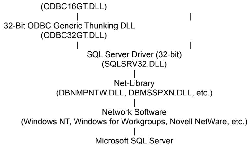
*Thunking* means intercepting a function call, doing some special processing to translate between 16-bit and 32-bit code, and then transferring control to a target function.
