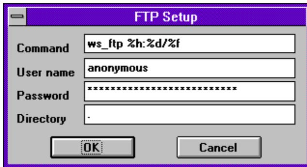
The command field should be tailored to give the full path name for the FTP program, e.g. "C:\FTP\WS\_FTP". The following special entries in this box will be substituted when an FTP request is made.
