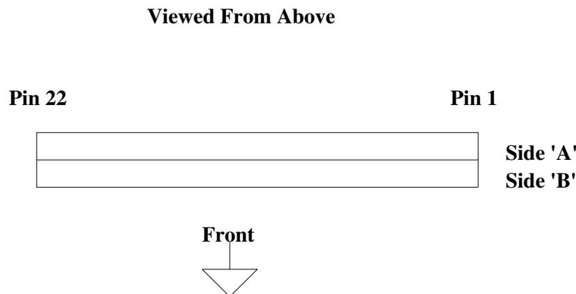
Cartridges are aligned and polarised by the case; they are plugged vertically into the host. All cartridges constructed to the time of writing have the components mounted on the pcb 'A' side.
