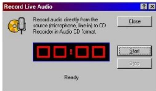
Clicking the Start button causes CD-Maker Deluxe to record the live audio data coming from your system's sound card and start recording it to disc. Simply click Stop to end the recording process.
