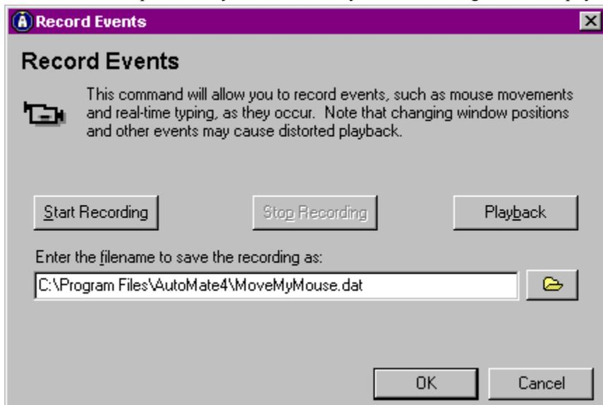
To record your mouse movements, first enter a filename and path of the file you would like to use to write the mouse movements to. Then, click the Start Recording button. AutoMate™ will minimize itself, and start recording the movements of your mouse and the keys you press. When you have finished, press Ctrl-Alt-F12. AutoMate™ will reappear, and your movements will have been written to the file.
