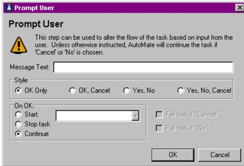
To setup the step, type in the text you wish to appear in the dialog box. Select which buttons you wish to be available by clicking an option in the Styles section.
