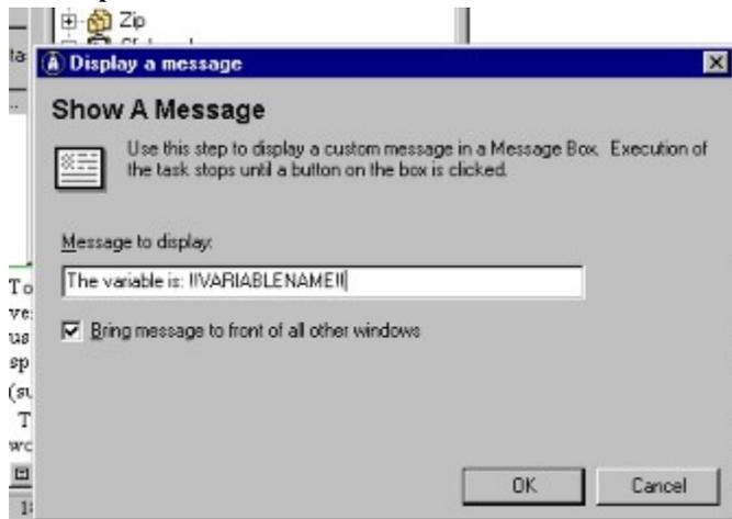
To use a variable, simply select it from within the [Step Builder](#) interface. Obviously, a variable is not very useful if data cannot be entered into it. When used in this way the task stops execution to ask for user input -- after the variable is populated with the users entry, other steps may reference the data by specifying the variable name anywhere in the step parameters, like this: `!!VARIABLENAME!!` (substitute VARIABLENAME for the variable name you used.)
