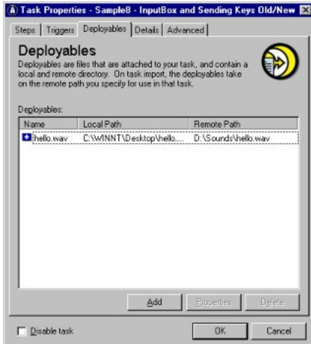
**Deployables:** Lists all the [Deployables](#) currently attached to this task. To modify or delete an item, highlight the item and select Properties or Delete.
