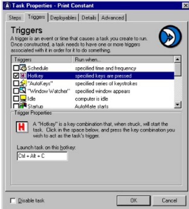
**Trigger List:** This is a list of available [triggers](#) for this task. To activate a trigger and set its properties, select the check box to the left of the trigger item in the list. Its properties will appear below.
