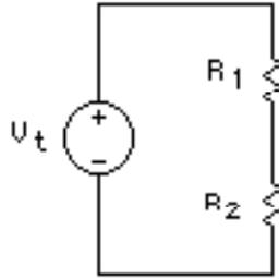
$$V_{R_L} = (V_t) \frac{R_{eq}}{R_1 + R_{eq}}$$
