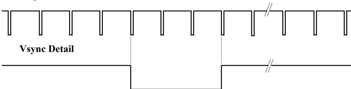
Note: Voltage levels to comply with EIA RS-343-A. H and Vsync are TTL level signals.
