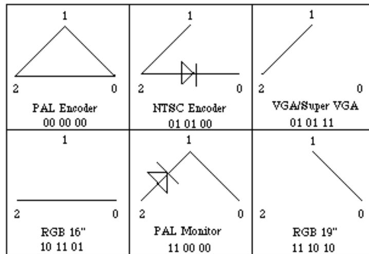
Figure 3 - Extended Type-7 Sense Line Decode Diagram
