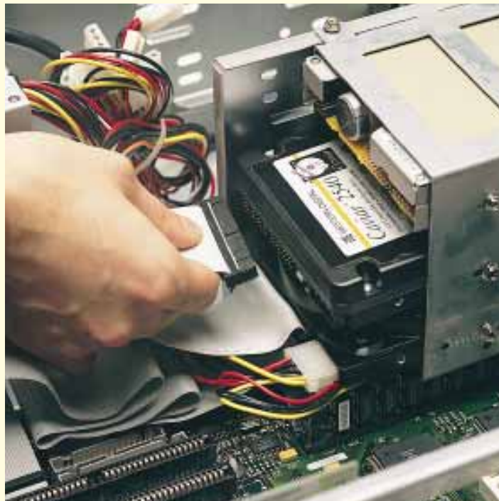
Connecting a Caviar 2540 IDE hard disk
