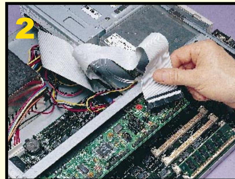
(1) Here, a new EIDE disk controller is fitted into place. This one is designed for a VL-bus
