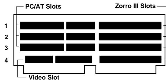
of XT or AT- style boards. The remaining Zorro III slots support both 24 & 32-bit Zorro boards.
