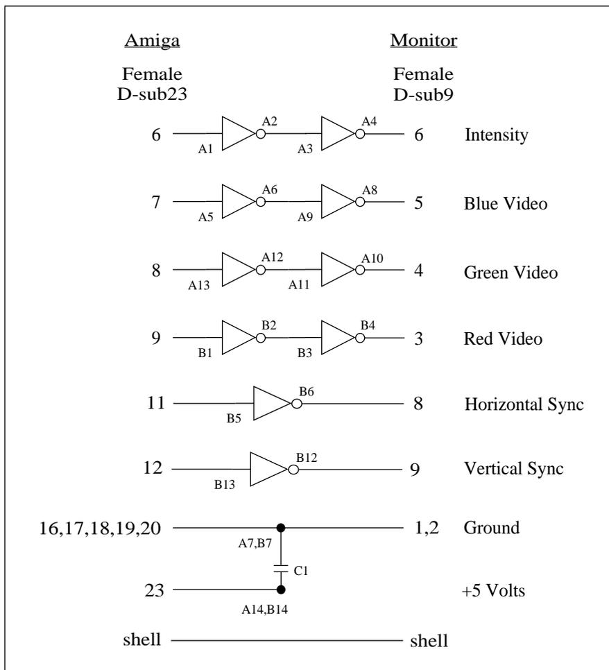
A1-A14 are pins 1-14 of a 74LS04 (hex inverter) IC chip. B1-B14 are pins 1-14 of another 74LS04 IC chip. C1 is a .1uf 16V ceramic capacitor.
