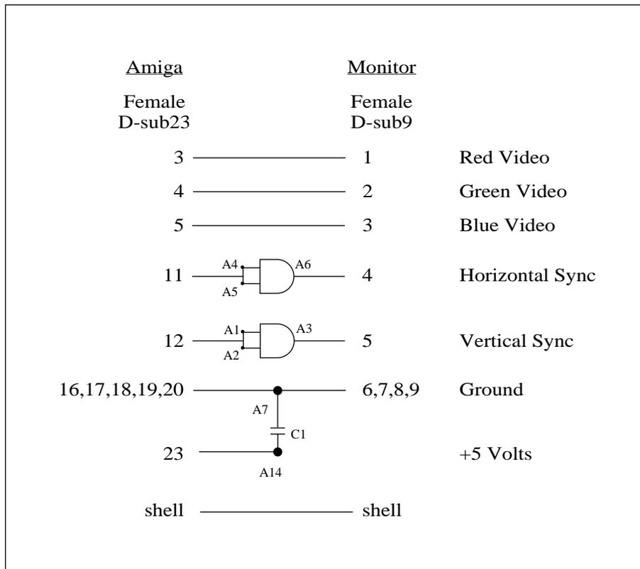
A1-A14 are pins 1-14 of a 74HCT08 (dual-input AND gate) IC chip. C1 is a .01uf 50V ceramic capacitor.
