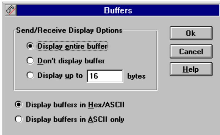
TracePlus will consume much more memory if you are tracing applications that send and receive data in large packet sizes (2048, 4096, etc.). To minimize memory usage, set a limit for buffer sizes, or turn off the buffer display altogether. Alternatively, you can set the trace buffer size to a smaller value, typically one half of the current buffer size.
