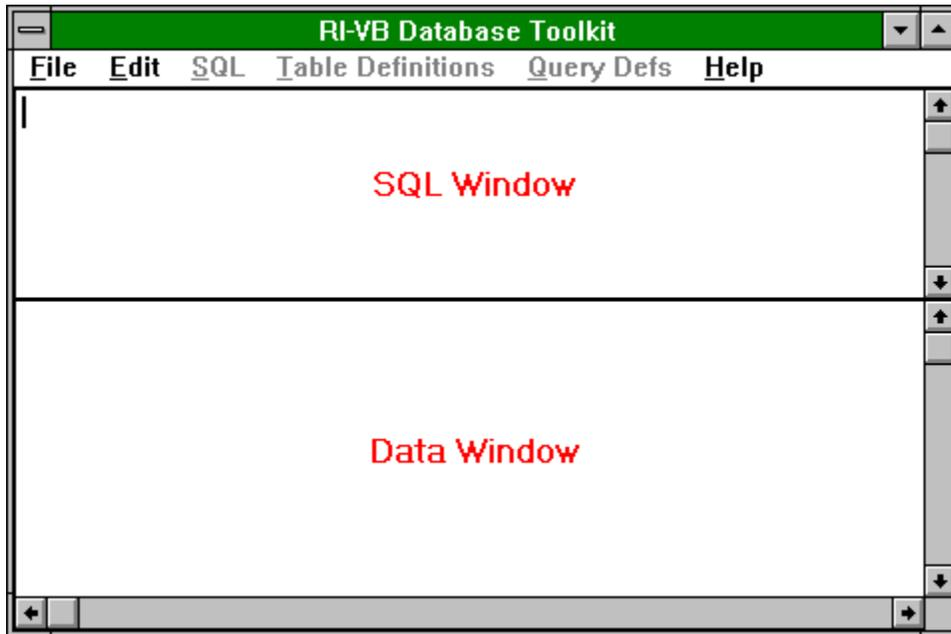
The lower two-thirds portion of the main window is called the Data Window. The output of the RI-VB Database Toolkit goes to this window where you can print, save to text file, and copy to the clipboard.
