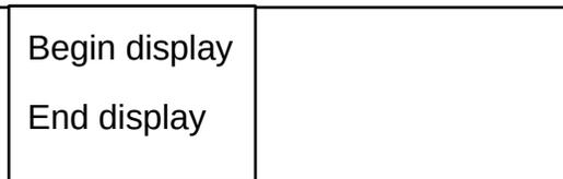
If arg1 of the WATCH() function is set to OFF, the Begin display option will be active and the End display option will be greyed. Select Begin display to show the script commands, as they are processed, in the client area. Conversely, if arg1 of the WATCH() function is set to ON, the End display option will be active and the Begin display option will be greyed.
