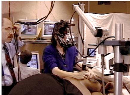
appear straightforward or even simple. It appears that all we must do is add a real-time rendering of ultrasound data to a live video background. However, realizing a working system requires addressing the technical problems of stereo AR, real-time volume rendering of time- and position-varying ultrasound data, and precise registration of real and synthetic image elements. In this section, we describe and justify our choice of technologies for various system components.
