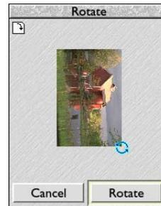
Ctrl O opens the **Rotate** dialogue. The dialogue is straightforward to use. Simply drag the thumbnail image. It will spin around its axis. As you rotate the image it will snap to the nearest 90 degrees. Release when it appears in the desired orientation. Click **Rotate** to effect the rotation.
