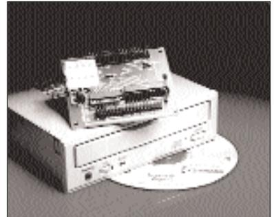
from the CD-ROM with that of the computer. The IDE-based drive, which is a double-speed multisession PhotoCD compatible unit, fits neatly into the Risc PC's standard 5.25 bay, and is accompanied by Clares ProArtisan 2CD and Cumana's own
