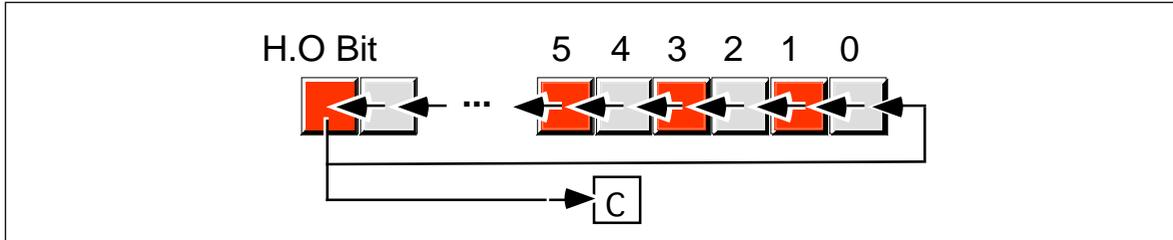
Figure 6.10 Rotate Left Operation
