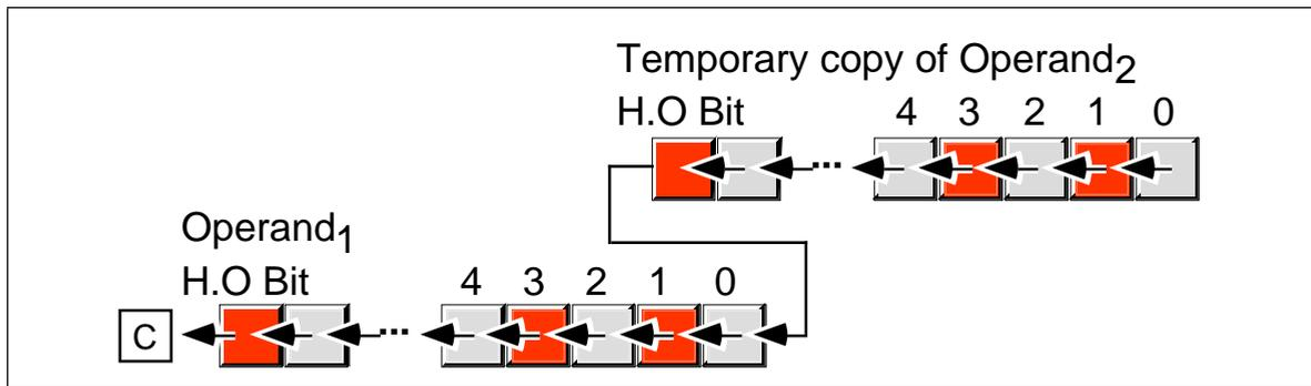
Figure 6.5 Double Precision Shift Left Operation
