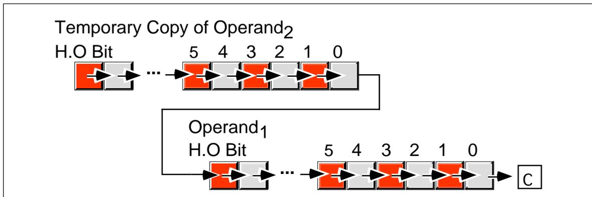
Figure 6.6 Double Precision Shift Right Operation
