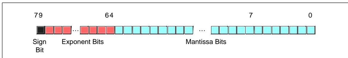
Figure 14.4 80 Bit Extended Precision Floating Point Format
