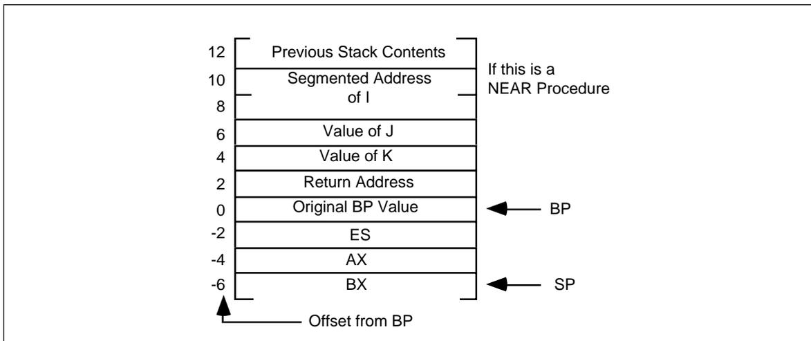
Figure 11.11 XYZ Stack Upon Procedure Entry
