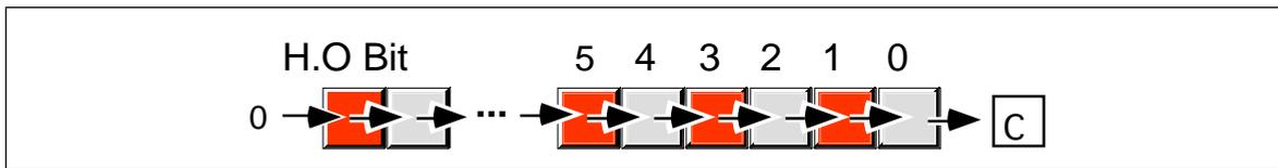
Figure 6.4 Shift Right Operation
