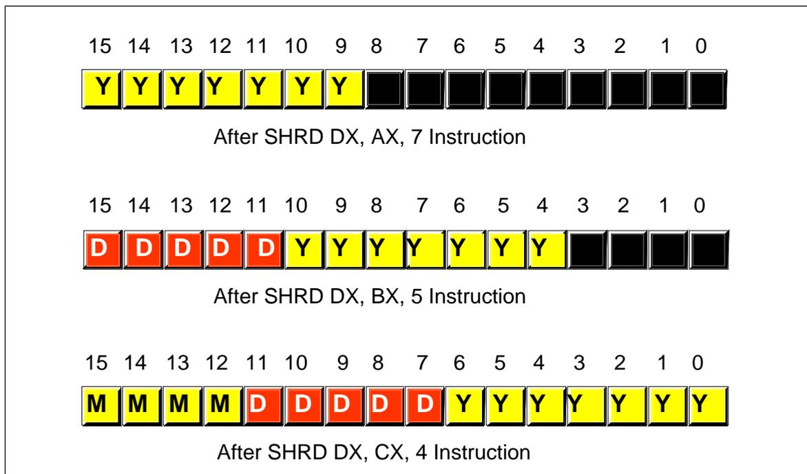
Figure 6.7 Packing Data with an SHRD Instruction
