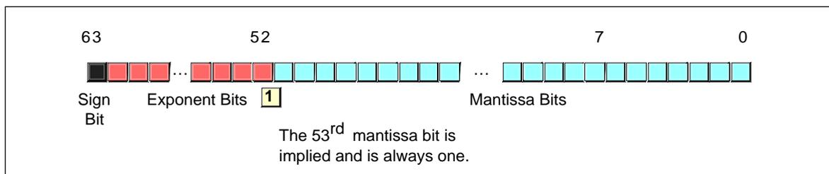
Figure 14.3 64 Bit Double Precision Floating Point Format
