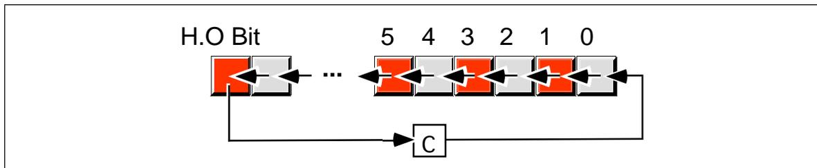
Figure 6.8 Rotate Through Carry Left Operation
