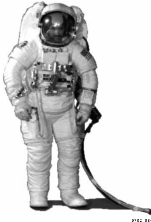
Figure 11-1. Extravehicular mobility unit
