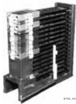
Figure 14-10. Intravehicular-charged particle directional spectrometer
