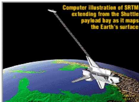
The [Shuttle Radar Topography Mission](#) objective is to demonstrate the technology for obtaining high-resolution digital topographic mapping of the Earth. SRTM consists of a specially modified radar system that will fly onboard the space shuttle Endeavour during an 11-day mission in early October 1999.
