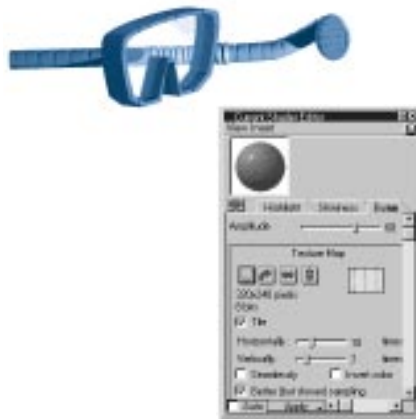
The indents on the snorkel were created by placing a texture map in the Bump channel
