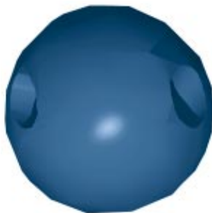
The object that results when you Boolean Subtract a bent pipe from a sphere.
