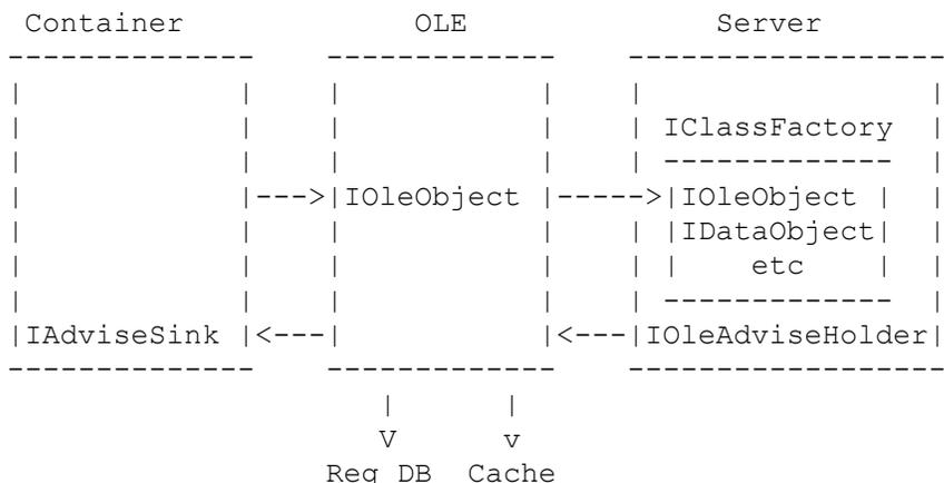
Note, the object still is not visible at this point. Now an explicit call to IOleObject::DoVerb() must be made with the verb OLEIVERB\_SHOW. This tells the server to make the object visible for editing.
