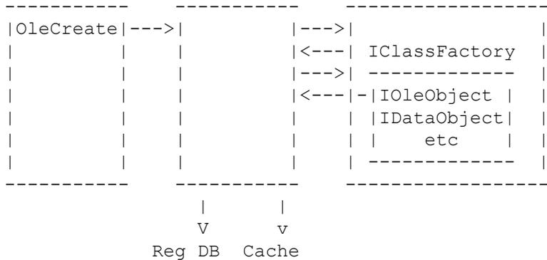
At this point, the creation routine returns to the container. Now, the container will generally query the interface pointer returned for the IViewObject interface. The container uses the IViewObject interface to ask the object to notify the container (through the container's IAdviseSink interface) every time the object's view changes, so that the container can update its display. At this point, the server creates an advise holder to notify the object of its changes:
