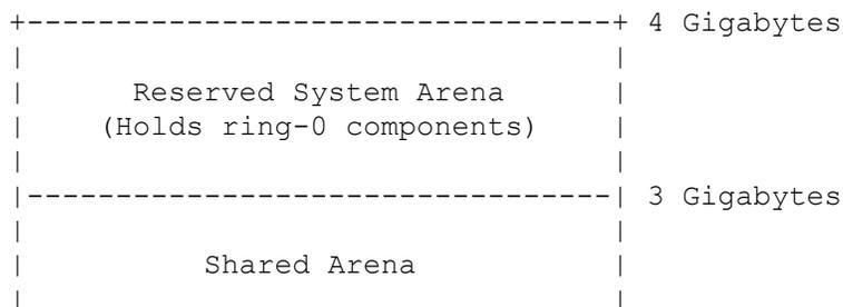
The shared arena is unique to Windows 95. This arena contains components that must be mapped into every process's address space. All of the pages in this arena are mapped identically in every process.
