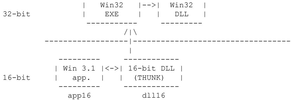
DLL16 is loaded when APP16 is loaded. DISP is spawned to handle WM\_COPYDATA messages, regardless of platform. DISP dispatches the calls to DLL32, marshalling the arguments.
