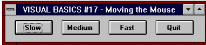
**VBEX017** moves the mouse up and down, left and right on the screen at various speeds. A control array of buttons is used to initiate mouse movement, and the index of the button pushed determines how many DoEvents() calls are put in the loop. The more calls, the slower the cursor movement.
