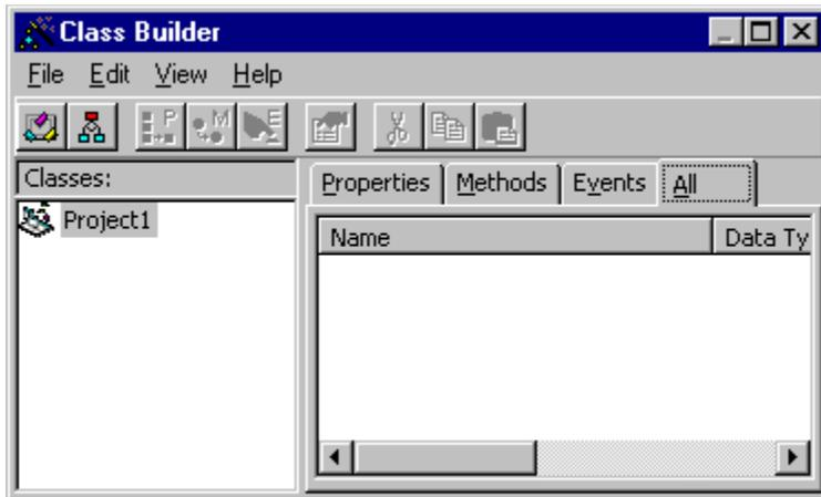
The Class Builder utility is meant to help you build your class and collection hierarchy for your Visual Basic Project. The Class Builder utility will keep track of the hierarchy of your classes and collections, and generate the framework code necessary to implement the classes and collections, including the properties, methods, and events.
