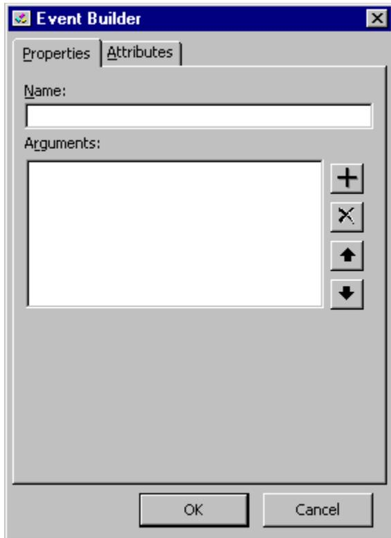
Allows adding a new event or editing an existing event of a class module. With this dialog box, the various properties and attributes can be specified for a new event or edited for an existing event.
