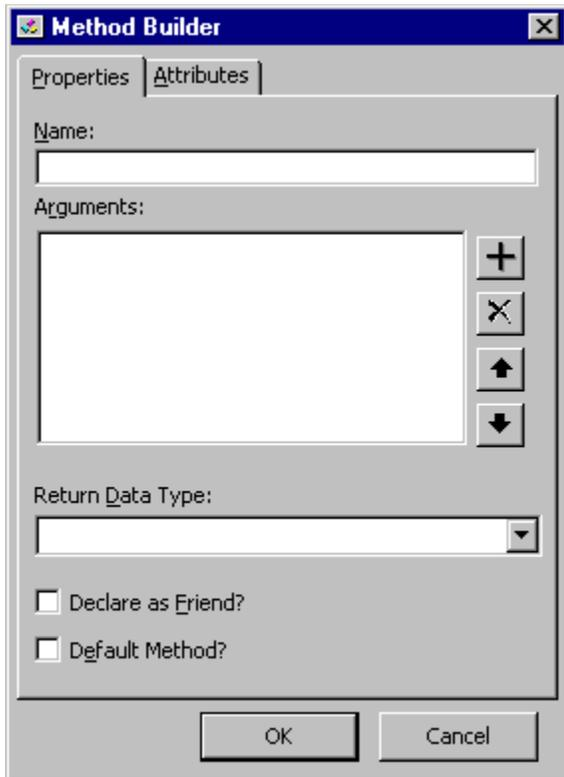
Allows adding a new method or editing an existing method of a class module. With this dialog box, the various properties and attributes can be specified for a new method or edited for an existing method.
