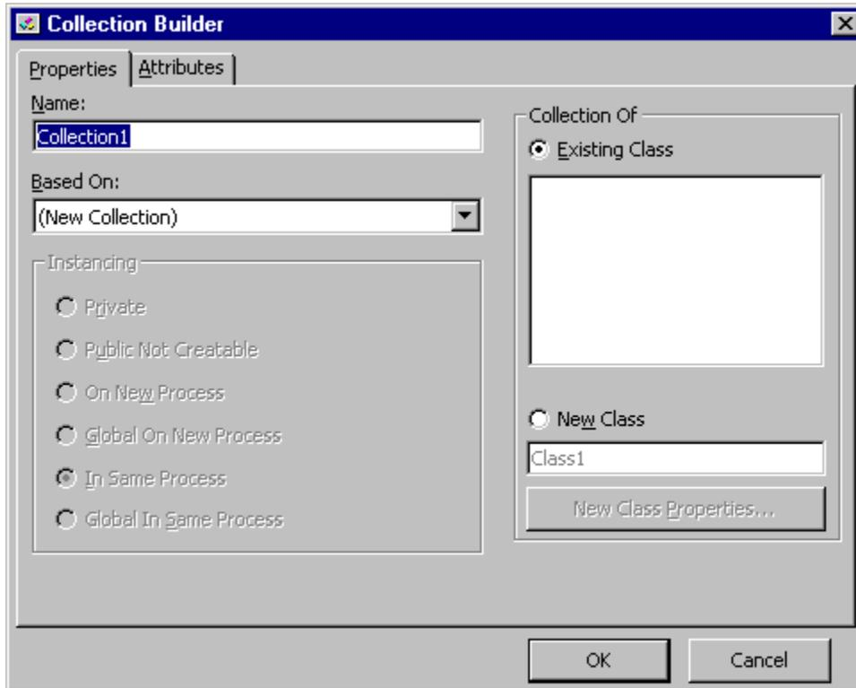
Displays and allows editing of the properties of the class module being added or edited.
