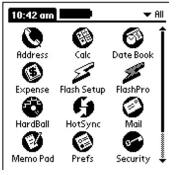
Use HotSync to install FPSetup.prc and FlashPro.prc to the Palm device. The icons FlashPro and Flash Setup should now appear.
