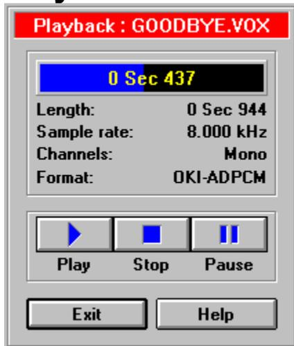
The playback window allows you to play the currently loaded file. This can be any file loaded using the File/Open menu commands or the result from the previous sound file conversion, if that file is still loaded. You can check which file is current by looking at the title bar. If the file name is Untitled, then no file is currently open. Otherwise, the title bar will give you the name of the currently open file. This file can be played by clicking on the Play button.
