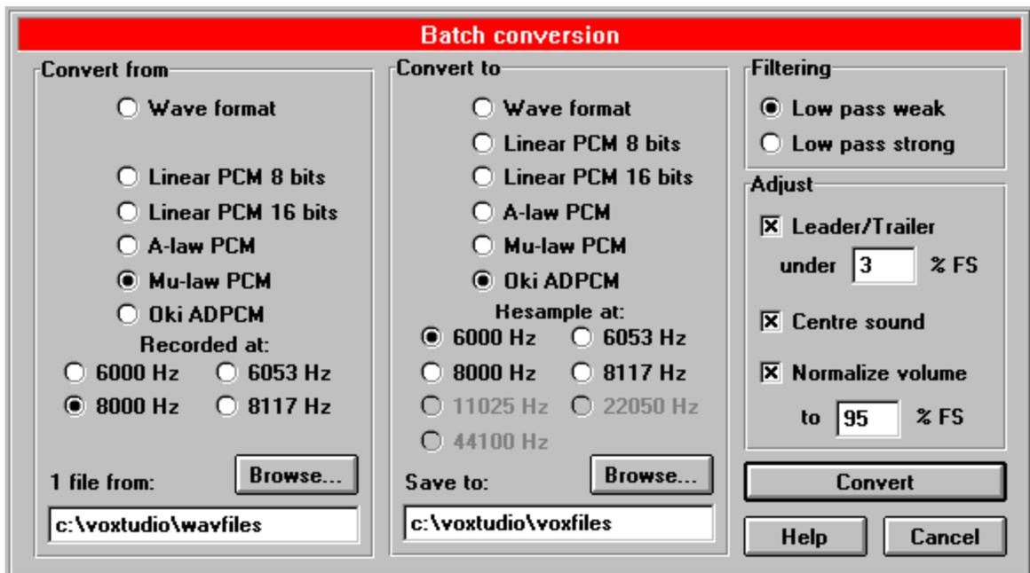
Select both a "convert from" and a "convert to" file format for batch conversions. The exact details of "convert from" files in wave ( .wav ) format need not be entered as Vox Studio reads that information from wave file headers. You do, however, need to specify the frequency for "convert to" wave formats. If the convert from format is a telephony format you need to give format details.
