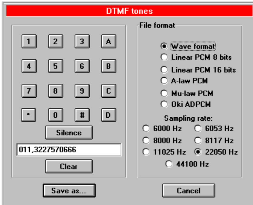
Compose a DTMF dial string on the keypad and save it in the desired file format. Avoid using 6 kHz sample rates for DTMF because of the inherently large frequency inaccuracies at such a low sampling rate.
