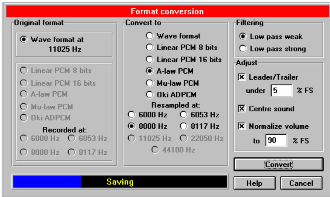
Select both a "convert from" and a "convert to" file format for manual conversion. The exact details of a "convert from" file in wave ( .wav ) format need not be entered as Vox Studio reads that information from the wave file header. You do, however, need to specify the frequency for a "convert to" wave format. If the convert from format is a telephony format you need to enter all format details.
