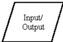
This symbol is used to represent information coming in and going out of the system, such as a customer order (input) or a product (output).
