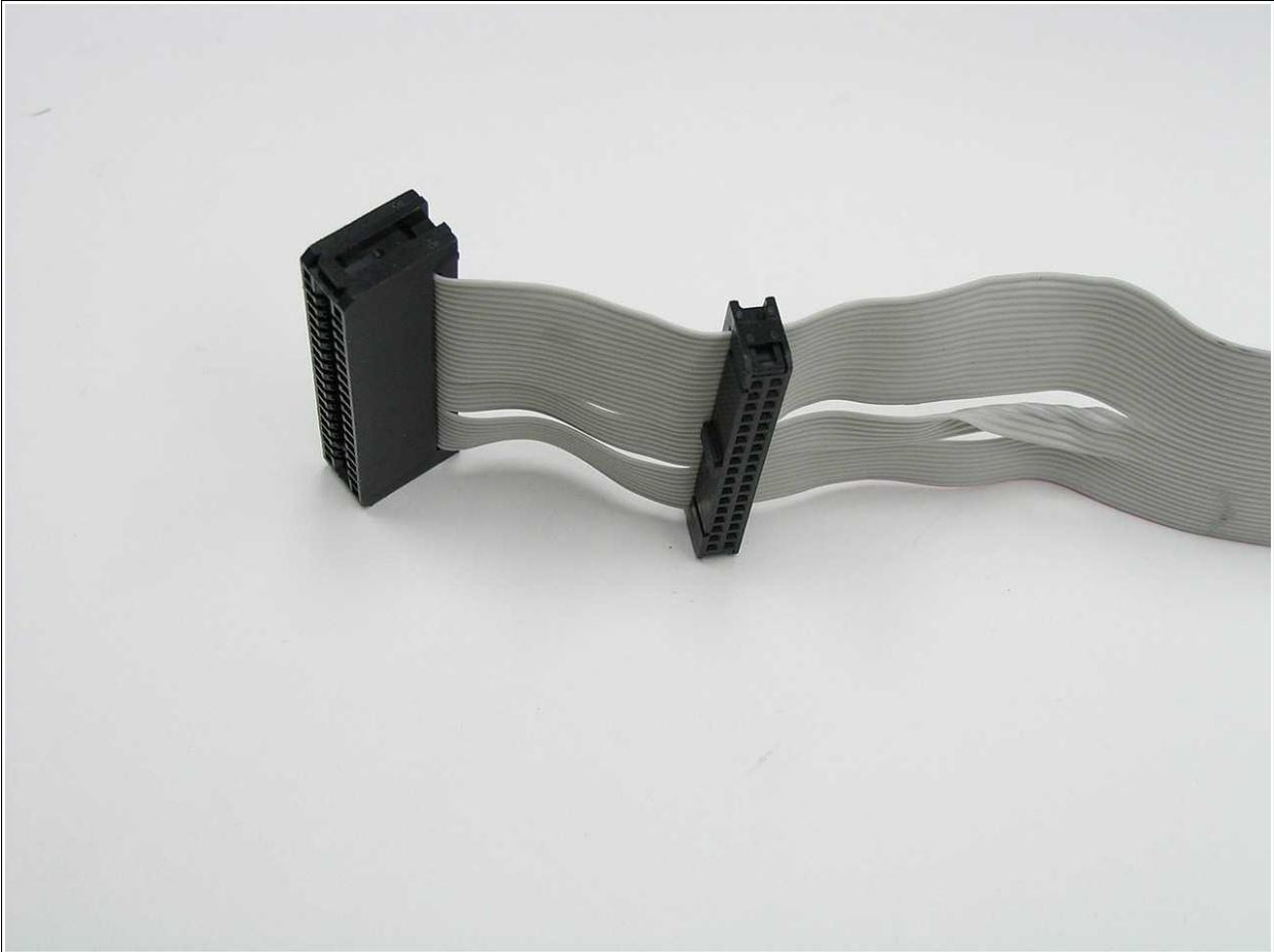
**Figure 5 – Connectors at the end of the cable are for Drive 0**
