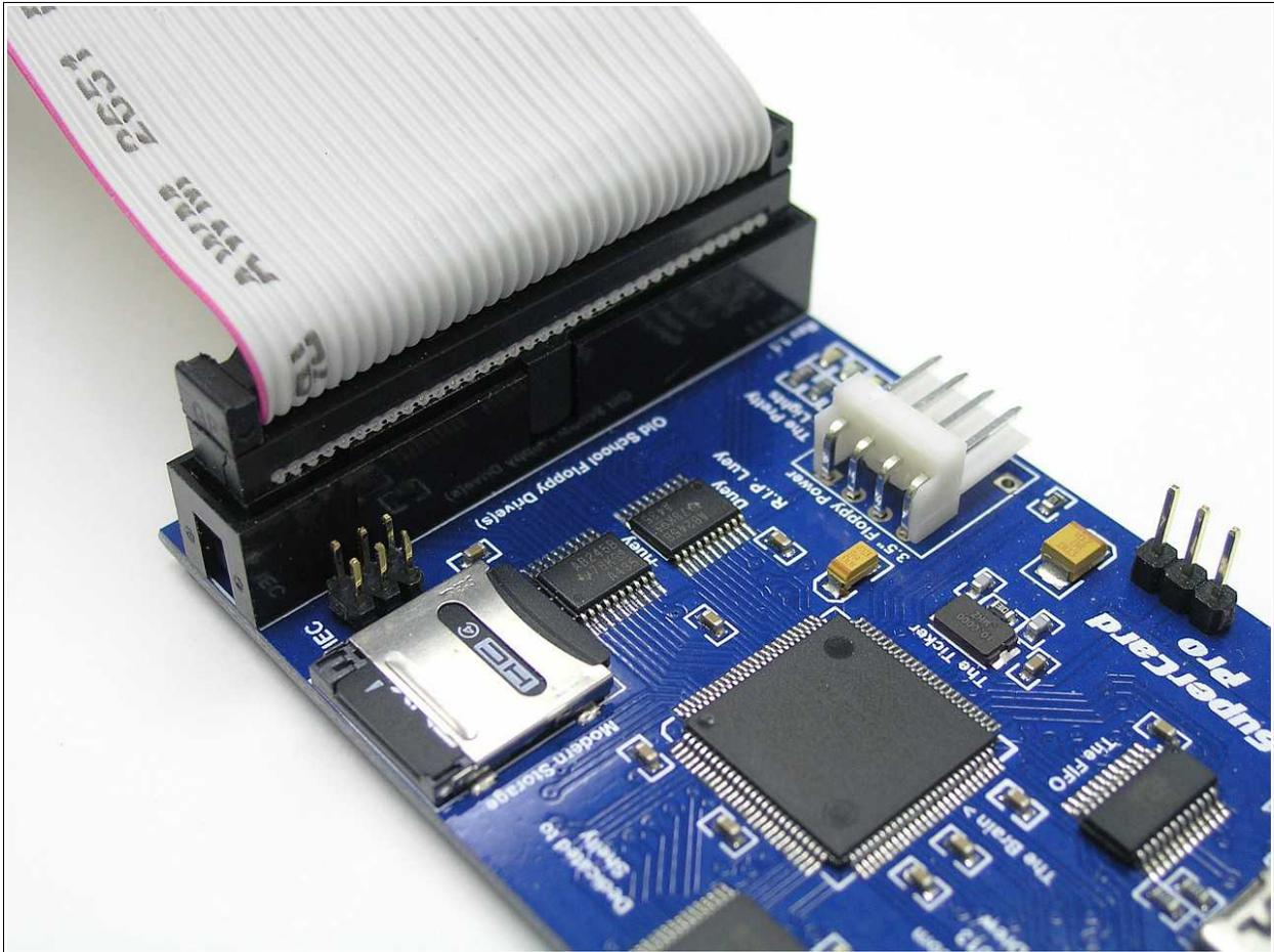
**Figure 2 – Floppy connector inserted into SuperCard Pro**
