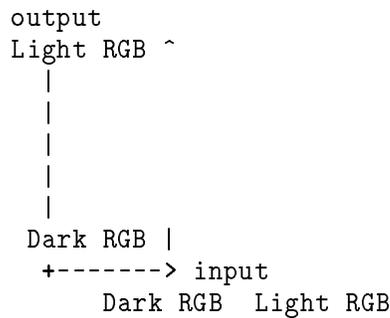
No operation is shown therefore with a straight diagonal line - the input value is mapped to the same output value.
