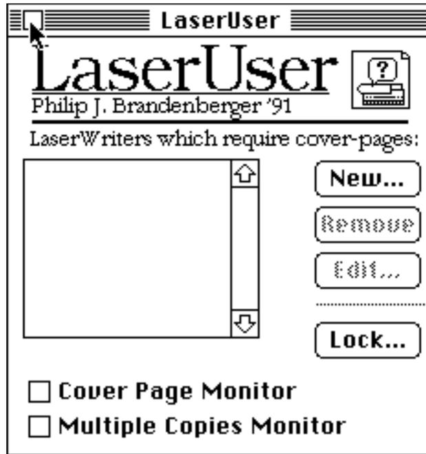
If the "Cover Page Monitor" box is unchecked, the cover-page settings in the application's "Print Of." dialog are left unchanged.
