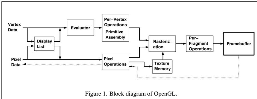
Figure 1. Block diagram of OpenGL.
