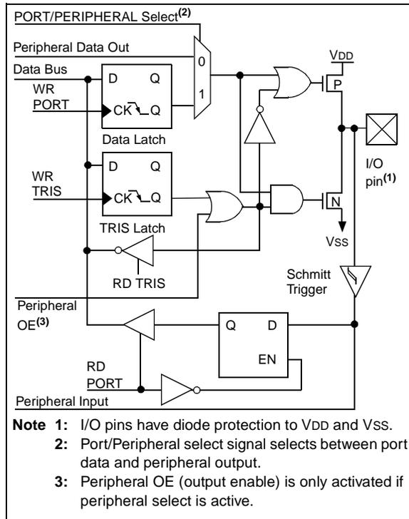
**FIGURE 3-6: PORTC BLOCK DIAGRAM (PERIPHERAL OUTPUT OVERRIDE) RC<3:4>**
