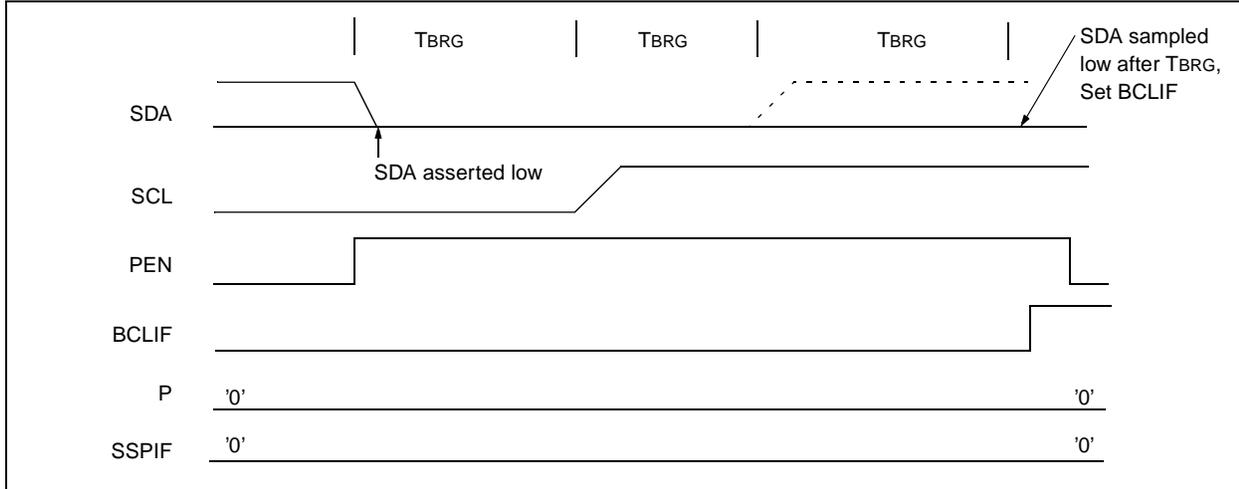
**FIGURE 9-26: BUS COLLISION DURING A STOP CONDITION (CASE 2)**
