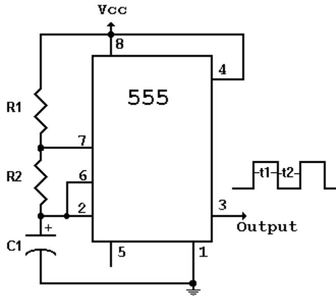
The astable or 'free-running' mode produces continuous output pulses. The frequency of the pulses (number of pulses per second) is determined by the components R1, R2 and C1. The formula
