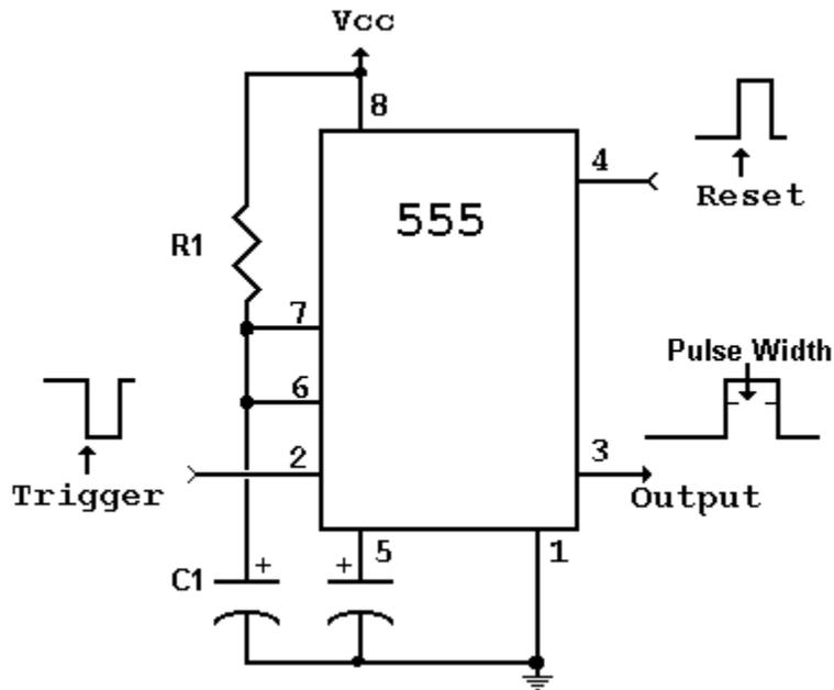
The monostable or 'one-shot' mode produces an output pulse for each negative going trigger pulse. The duration of the output pulse is determined by the timing components R1 and C1. The formula used is  $t = R1 \times C1$ . The voltage value of the pulse is approximately  $\frac{2}{3} V_{cc}$ .
