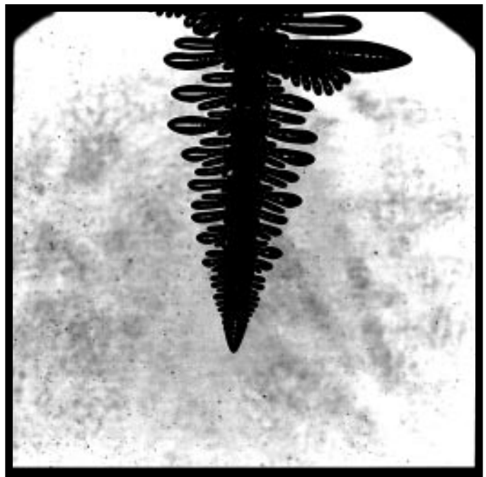
Figure 21. A dendrite grown in the Isothermal Dendritic Growth Experiment (IDGE) aboard the USMP-2. This is an example of how most metals solidify.
