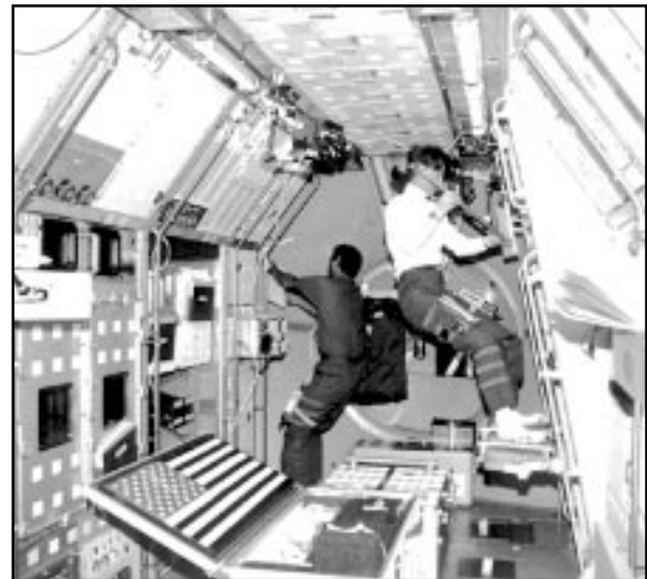
Figure 19. Astronaut Bonnie J. Dunbar, USM-1 payload commander, is about to load a sample in the Crystal Growth Furnace as payload specialist Lawrence J. DeLucas, at the multipurpose glovebox, confers with her.
