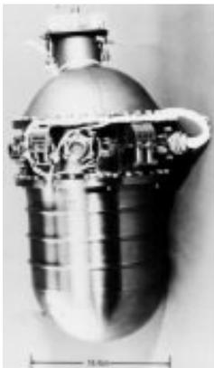
The composition of the atmosphere of Jupiter had been studied intensively with ground- and space-based observations, but many questions remained. The neutral mass spectrometer (NMS) was designed to provide a detailed analysis of the chemical composition of the atmosphere and aid in understanding the processes responsible for the complex, colorful clouds.
