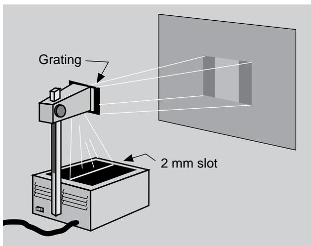
of visible light are bent different amounts and this causes them to be dispersed into a continuum of colors. (See diagram.)
