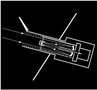
**Description:** The principle of a reflector telescope is demonstrated with a concave makeup mirror.
