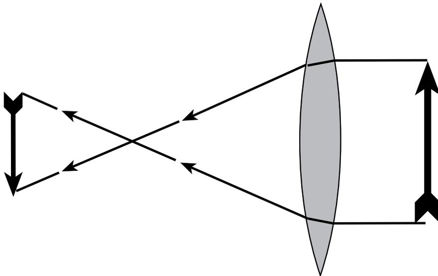
Images seen through lenses, such as this double convex lens, are inverted. This is similar to the function of the pinhole in the pinhole viewer.
