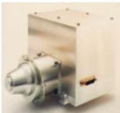
Pioneer and Voyager spacecraft passing by Jupiter measured radiation leaving Jupiter's cloud tops, but we could only guess about the nature of radiation within the atmosphere. In contrast, the net flux radiometer (NFR) in the probe was designed to directly sample the local energy flows within and below the Jovian cloud layers.
