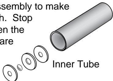
With a small amount of effort, the assembly will compress slightly and slip inside the tube. (Do not insert them yet.) Friction will hold them in place. If the lens assemblies get too loose, they can be held firmly with glue or tape.
