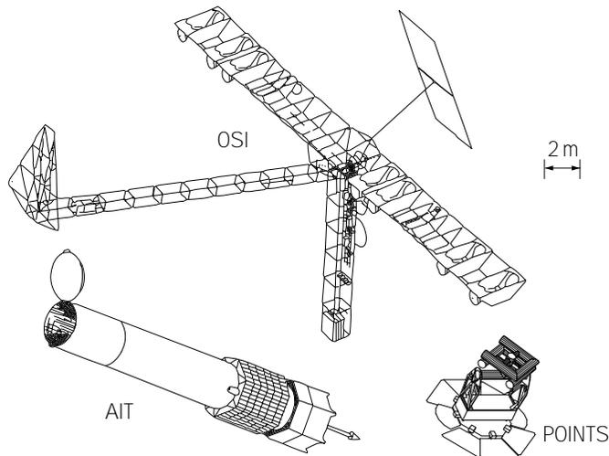
*Figure 3-11. The three candidate instruments for implementation during TOPS-1: the Astrometric Imaging Telescope (AIT), the Precision Optical Interferometer in Space (POINTS), and the Orbiting Stellar Interferometer (OSI). The systems are drawn to scale with the reference mark for 2 meters shown in the figure.*
