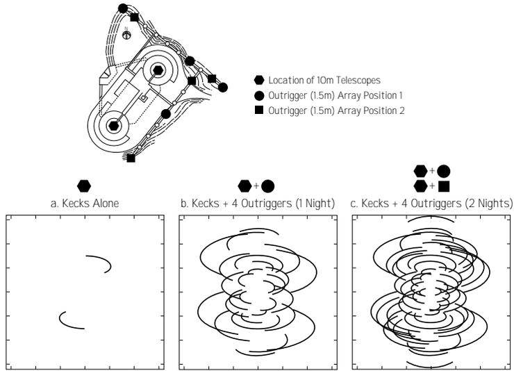
Figure 4-19. *U-v coverage available with the Keck Interferometer.*
