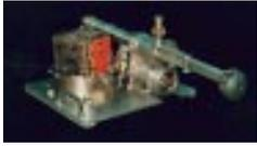
The nephelometer (NEP) was used to investigate the structure of clouds and the characteristics of particles in the atmosphere of Jupiter. (In Greek, the word “nephelē” means “cloud.”) Knowledge of cloud properties allows modeling of the paths of energy balance for Jupiter.
