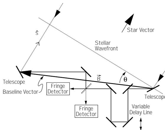
Figure 3-10. Astrometry with an interferometer. The delay at which fringes are observed is  $\vec{B} \cdot \hat{s} + C = |\vec{B}| \sin \theta + C$ .
