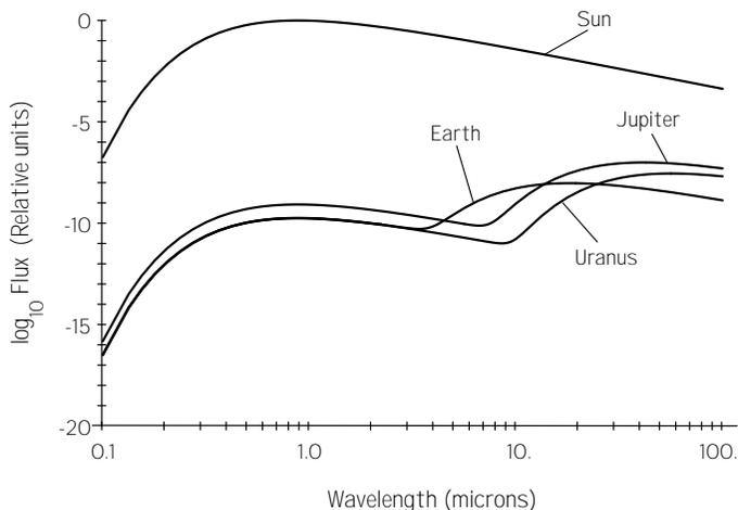
*Figure 4-1. The spectral energy distributions of the Sun, Jupiter, Earth, and Uranus as they would appear at 5 pc, averaged over a 10% spectral bandpass. Note the decreased ratio of solar to planetary flux in the thermal infrared, compared to visible wavelengths.*
