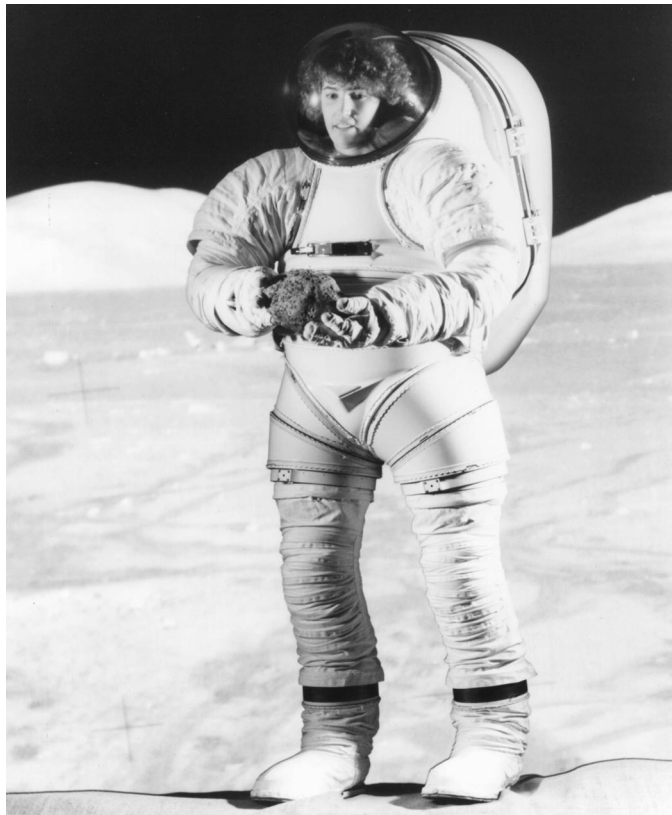
The ZPS Mark 3 spacesuit has a metal upper torso and a hard metal brief connected with a rolling waist joint. The waist joint has sizing rings so torso length can be adjusted to fit different size crew members.
