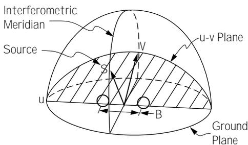
*Figure 4-8. Representation of the  $u$ - $v$  plane for a Michelson interferometer. In this case, the source is in a direction perpendicular to the interferometer baseline  $B$ . The  $u$ - $v$  plane is constructed normal to the observing direction.*
