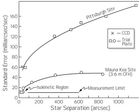
Mauna Kea are plotted in Figure 3-8, which shows the relative image motion of star pairs as a function of their separations. A least-squares fit to these data in the analytic form of Equation (3.5) yields  $\sigma_\theta = 0.054$  arcsec and  $a = 0.35$ .
