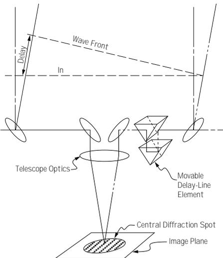
*Figure 4-7. A Michelson interferometer in the image plane version. The incoming rays are reflected off plane mirrors, and the diffraction spots are merged by the optics of a telescope (a lens is shown, but a set of reflecting optics works as well). The two beams alternately interfere destructively or constructively, giving fringes in the image plane. The path lengths are equalized by delay line optics.*
