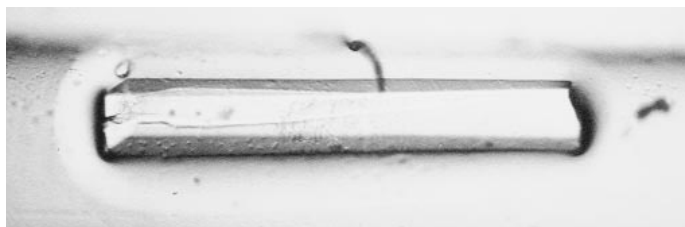
This crystal of the Factor D protein was grown on the USML-1 mission.
