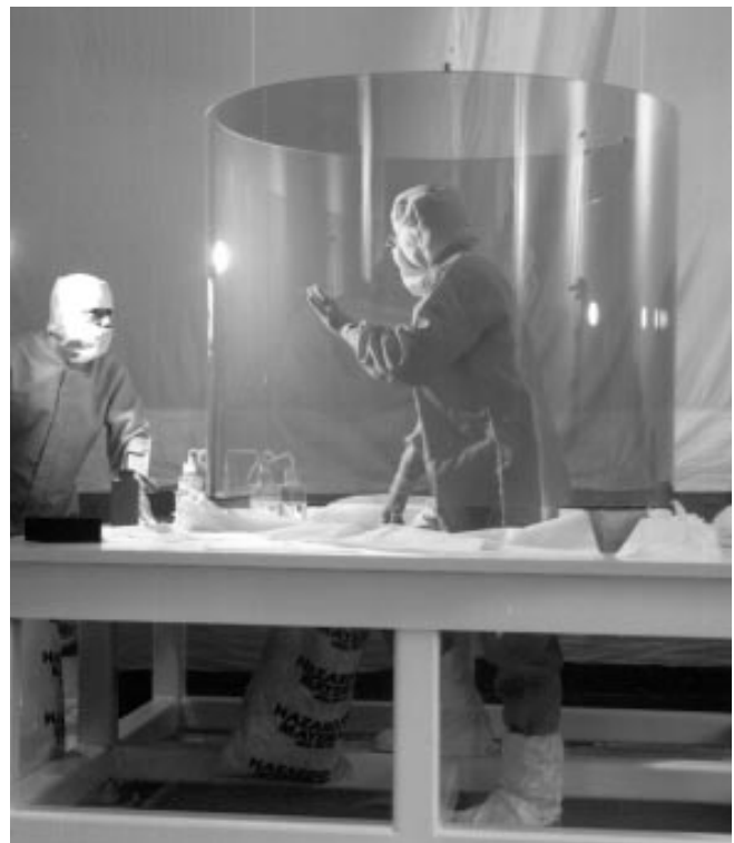
Quality inspectors perform a visual inspection of the P1 (Parabola 1) optic for NASA's Advanced X-ray Astrophysics Facility (AXAF). P1 measures 1.2 meters in diameter by 1 meter in length and weighs 520 pounds. The wall of the optic is only nine tenths of an inch thick. All eight AXAF mirrors will be completed by Spring 1995; an end-to-end x-ray test of AXAF will be conducted starting in January 1997. (Hughes-Danbury Optical Systems)
