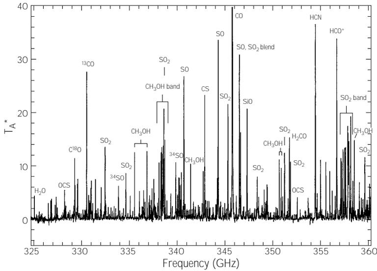
*Figure 4-4. The spectrum of the core of the Orion star-forming cloud in the 0.9 mm wavelength band. The vast numbers of spectral lines are diagnostic of different conditions of density and temperature throughout the nebula. High-resolution aperture synthesis maps made in different molecular lines will provide detailed information about the physical and chemical properties of the region.*
