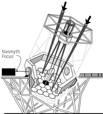
Figure 4-12. Keck telescope optical configuration and focal positions.
