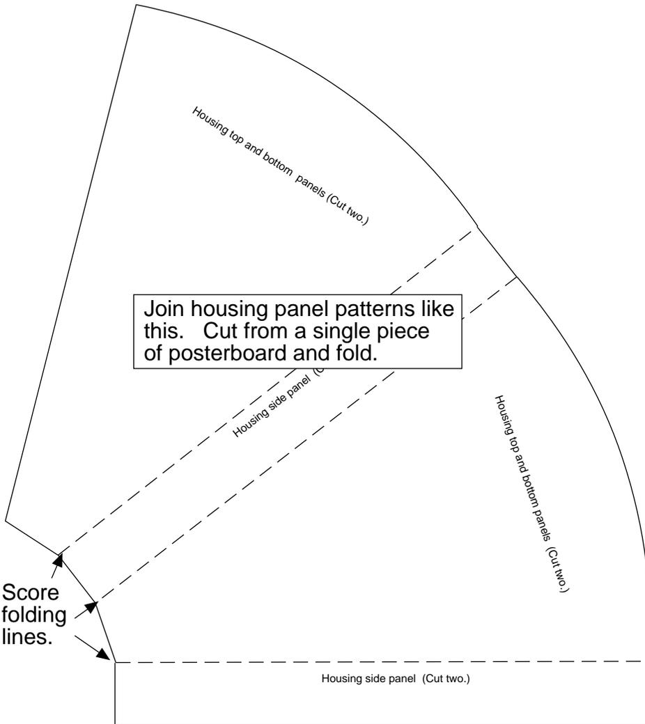
Join housing panel patterns like this. Cut from a single piece of posterboard and fold.
