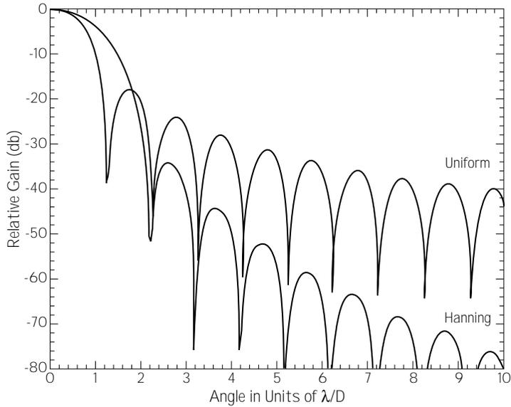
*Figure 4-5. The radial dependence of the unblocked aperture (i.e., uniform illumination) compared to the pattern for a Hanning taper (apodization). The response is logarithmic (10 db = one factor of 10); note the dramatic reduction in the far pattern of the tapered response. The increased width of the principal response should also be noted.*
