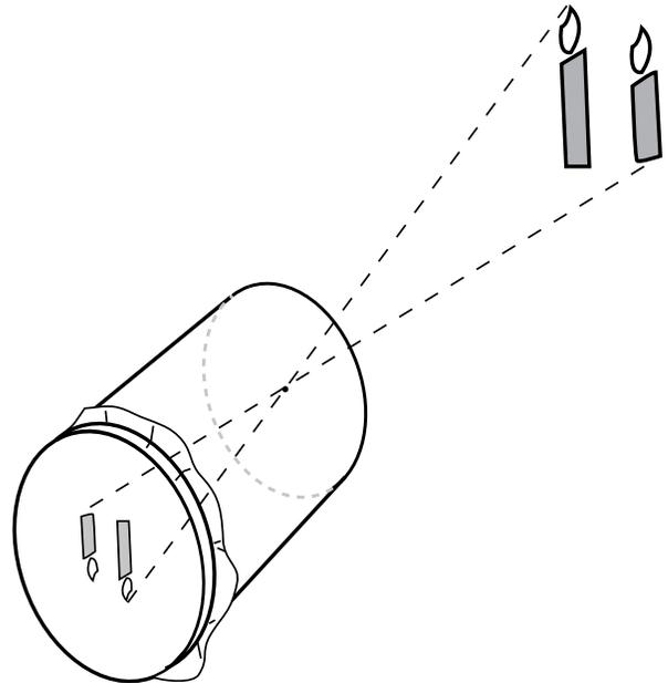
becomes inverted. (See diagram on next page.) With the pinhole viewer, the change takes place at the pinhole.
