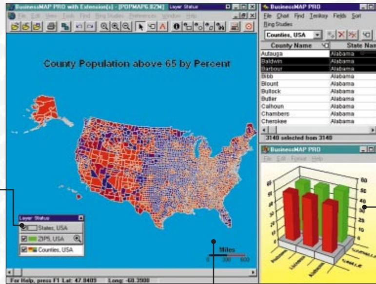
Floating Layer Status Bar controls viewing and drawing order of map layers. Magnifying glass indicates layers visible only at zoomed in scale.
