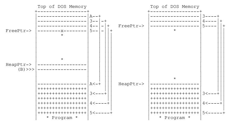
TEGL uses the more efficient method of maintaining the free space chain in sorted order. This allows allocation of memory to favor the lower portion of the heap. This does not remove the fragmentation problem where one non-movable records is allocated in the middle of the heap.
