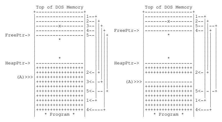
If adjacent memory is found, the free space pointer is removed from the freeptr chain and TEGL's heap manager takes the most recent entry and moves it to fill the now empty position. The size and the original pointer (A) is adjusted to reflect a new pointer position and size.
