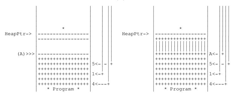
When all possible adjacent blocks have been removed, the TEGL heap manager checks if the end of memory block is equal to the heapptr. If not, a free space entry is added to the bottom of freeptr.
