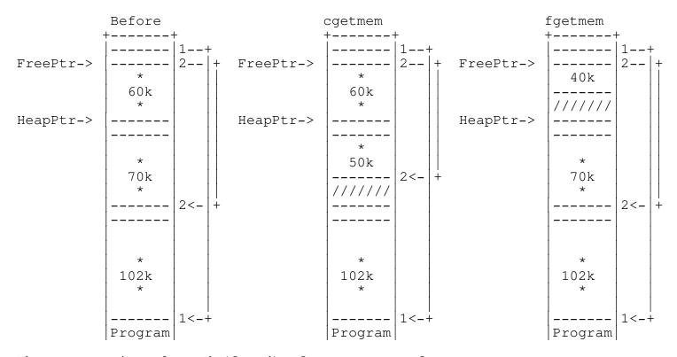
When memory is released (freed), fgetmem uses cfreemem to release the memory block back into the heap.
