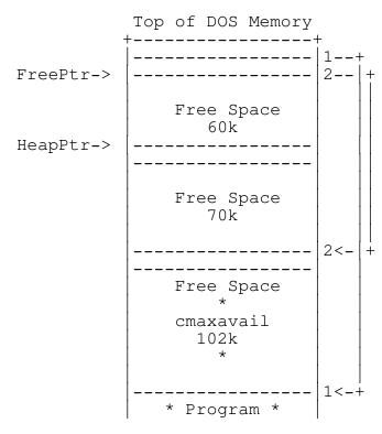
When memory is requested from the TEGL Heap Manager, a sequential scan of the freeptr chain is made to see if any of the free memory space can be re-used. Any free space that satisfy the requested size will be used.
