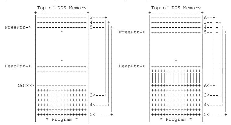
When all possible adjacent blocks have been removed, the TEGL heap manager checks if the end of memory block is equal to the HeapPtr. If not, a free space entry is added to the bottom of FreePtr.
