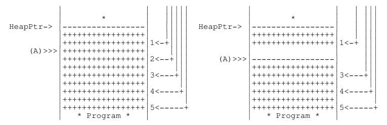
If adjacent memory is found, the free space pointer is removed from the FreePtr chain and TEGL's heap manager moves the free chain structure up by one entry to close the empty position. The size and the original pointer (A) is adjusted to reflect a new pointer position and size.
