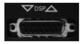
All NeXT computers include a digital signal processor (DSP) port providing direct input/output to the Motorola DSP56001 chip on the NeXT computer's CPU board. This port can accept digital input from lab-
