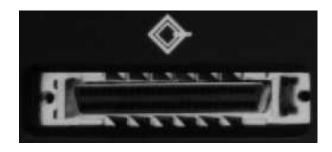
NeXT computers implement the SCSI-1 protocol using a SCSI-2 connector. When the SCSI-2 protocol is fully defined, NeXT will implement and support it. Until then, NeXT will be compatible with all existing SCSI-1 devices. NeXT also provides cables connecting SCSI-1 and SCSI-2 connectors.
