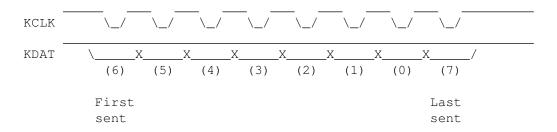
The keyboard processor sets the KDAT line about 20 microseconds before it pulls KCLK low. KCLK stays low for about 20 microseconds, then goes high again. The processor waits another 20 microseconds before changing KDAT.
